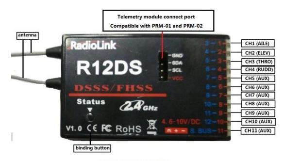
PWM signal working mode: Red LED, output 11 channels PWM signal
