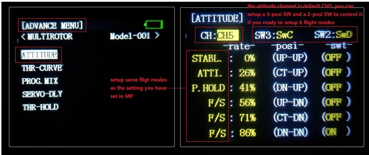
3. Setup Flight Mode 1 is Stabilize both in Mission Planner and transmitter. Make sure the -swt- is ON (by press the 3 Posi-SW or 2 Posi-SW to make it ON or OFF) and then you can setup the PWM data. Setup the PWM value according to the default numerical interval (change the value by turn the dial, press the Push button when you choose the right value.
