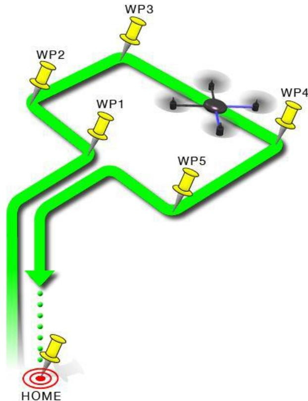
AUTO mode incorporates the altitude control from AltHold mode and position control from Loiter mode and should not be attempted before these modes are flying well. All the same requirements apply including ensuring that vibration levels and compass interference levels are acceptable and that the GPS is functioning well including returning an HDOP of under 2.0.
