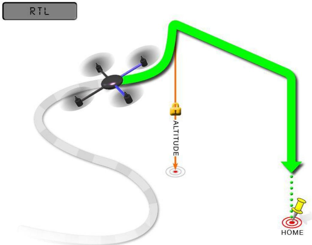
RTL is a GPS-dependent move, so it is essential that GPS lock is acquired before attempting to use this mode. Before arming, ensure that the APM's blue LED is solid and not blinking. For a GPS without compass, the LED will be solid blue when GPS lock is acquired. For the GPS+Compass module, the LED will be blinking blue when GPS is locked.
