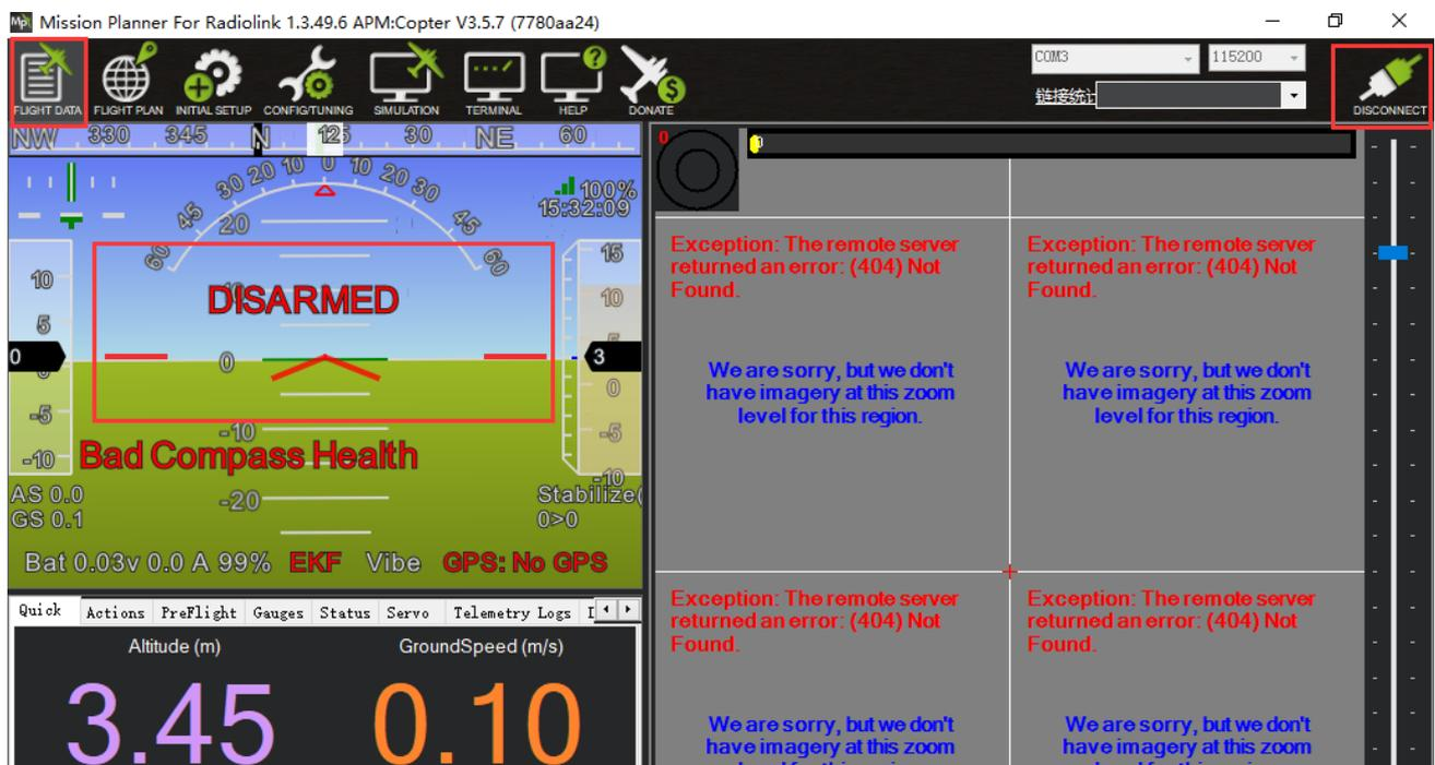
Under Initial Setup--Mandatory Hardware--select Accel Calibration from the left-side menu--Click Calibrate Level to start the calibration.
