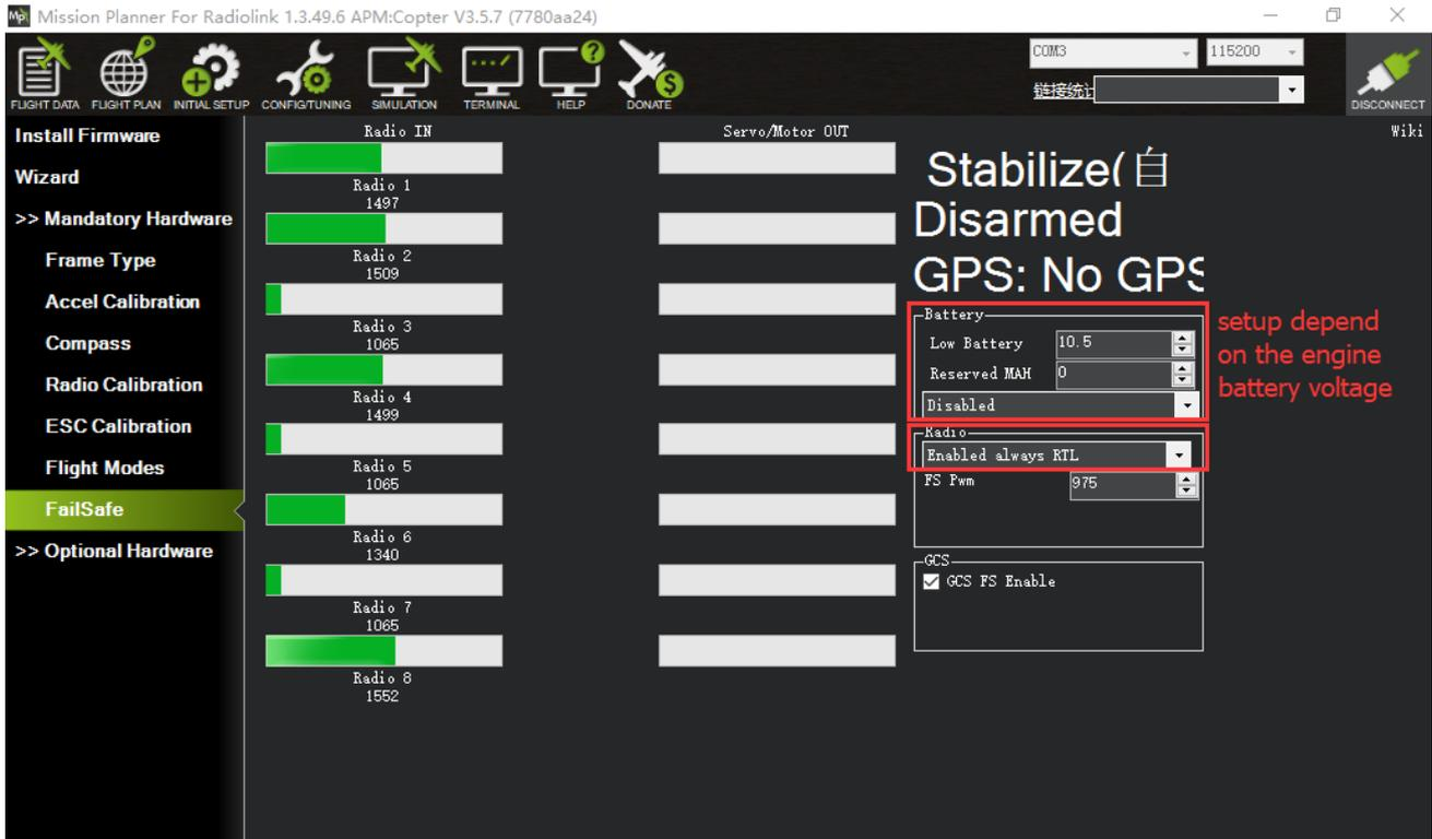
You can turn off transmitter to check if the Failsafe function setup success(the PWM of CH3 is smaller than 975)
