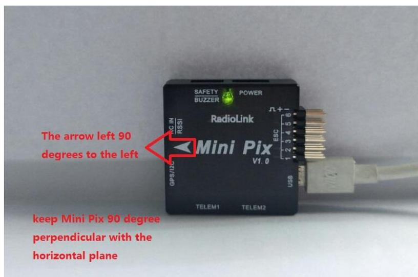
3. Place vehicle on its RIGHT side and press any key to save setting.
