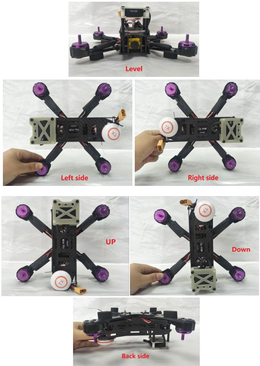
8. When there are three D sounds made by the buzzer, it means the compass calibration is done with success. Restart the flight controller and it's enabled.
