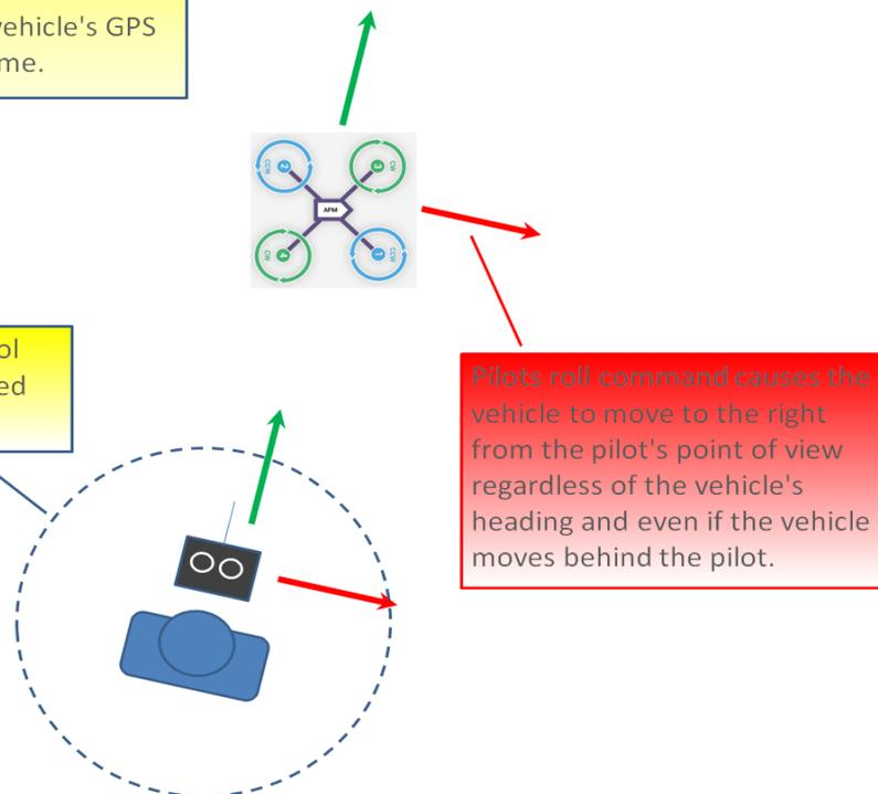
Super Simple mode is the same as simple mode except that it uses the vehicle’s position relative to home instead of the vehicle’s initial heading when it was armed. This means that no matter where the vehicle is, pulling the pitch back will cause it to return towards home regardless of the vehicle’s actual heading.
