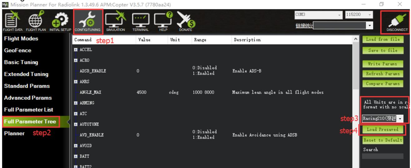
Reset to default: reset all the parameters to default files. Please recalibrate and re-setup all the parameters after reset.
