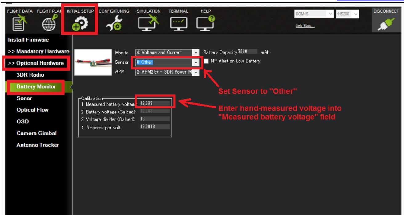
Using the power analyzer you can also measure the current and compare to results displayed in the Mission Planner.
