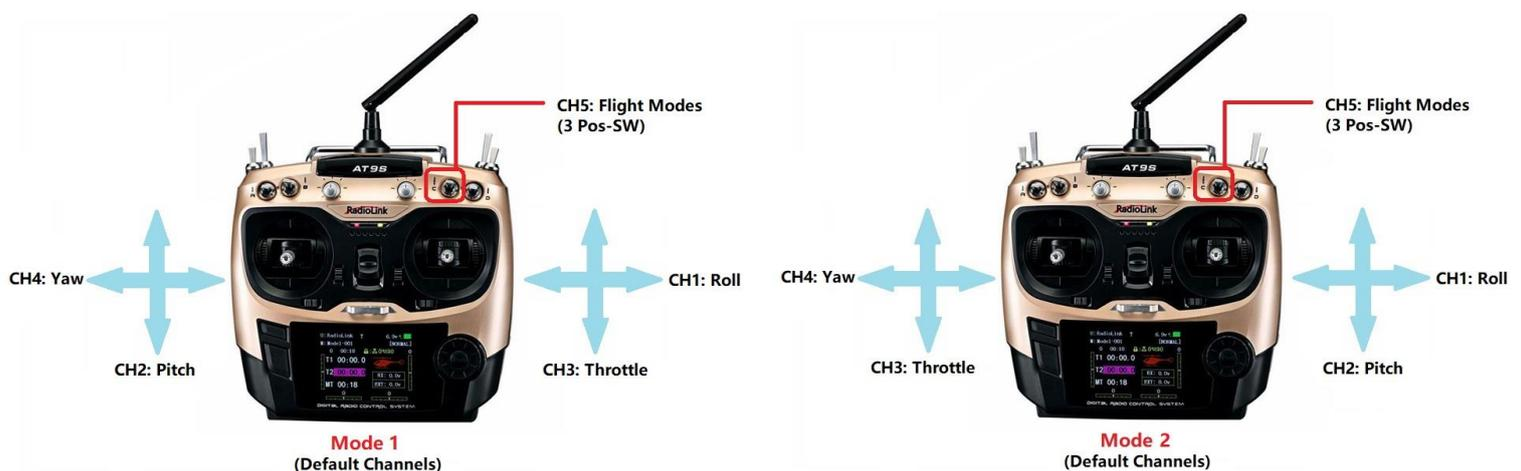
For safety, you should disconnect the battery and/or remove propellers before performing radio calibration. Bind your transmitter and receiver before calibrate radio, connect MINI PIX to computer via USB cable and then turn on transmitter. The RC receiver ask to connect to the RC port of MINI PIX.
