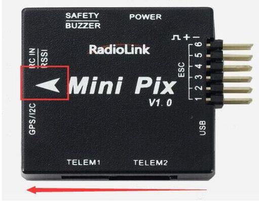
Keep the GPS with the same direction of MINI PIX if you need to use MINI PIX with GPS.
