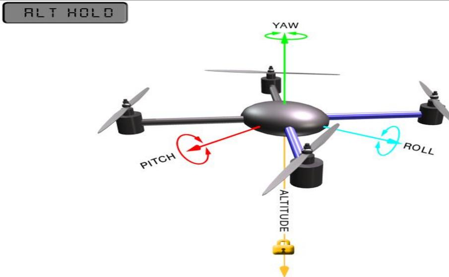
**Note:** The flight controller uses a barometer which measures air pressure as the primary means for determining altitude (“Pressure Altitude”) and if the air pressure is changing in your flight area due to extreme weather, the copter will follow the air pressure change rather than actual altitude. When fitted and enabled, a downward facing rangefinder such as LiDAR or SONAR will automatically provide even more accurate altitude maintenance, up to the limit of the sensor.
