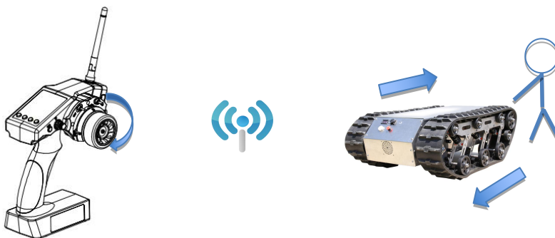
Steering mix throttle setup completed, left track moves forward while right backward when turning the wheel clockwise. The differential realizes the right turning of track vehicle
