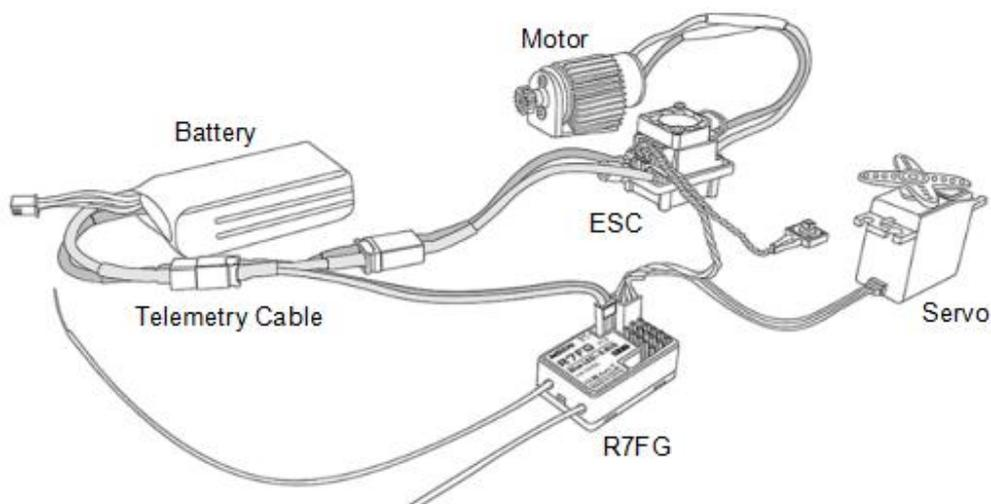
When connect with success, users can check the battery voltage on the main interface of the transmitter.
