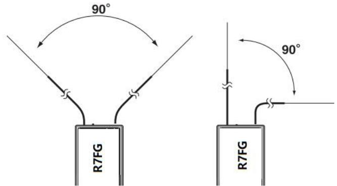
3. Big models may contain metal parts that influence signal emission. In this case, antennas should be positioned at both sides of the model to ensure the best signal status in all circumstances.
