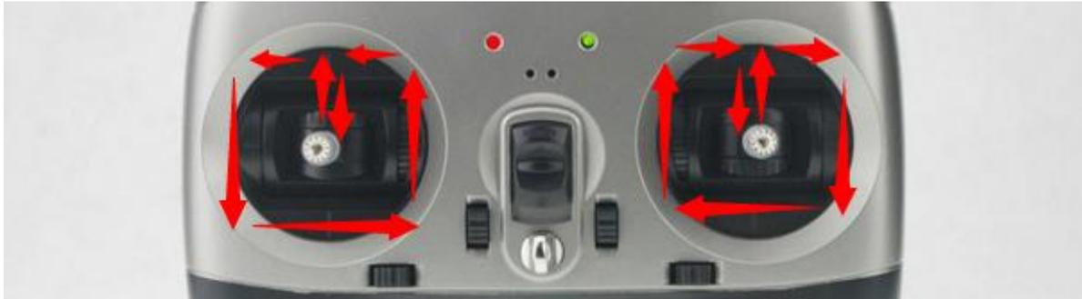
If the green bars do not change when pilots toggle the sticks, please check if the receiver has connected successfully. Also, check if every corresponding green bar for every channel works as listed:
