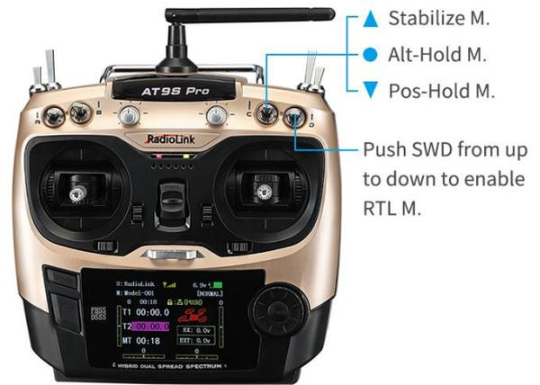
2. When flight mode 1 in MP is Stabilize, the first ATTITUDE on transmitter should be set as Stabilize and the corresponding parameters setup in MP should be set as below:
