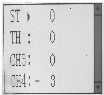
1. Enter the function menu and use “Dec(-)” or “Inc(+)” button to access SUBTR function.
