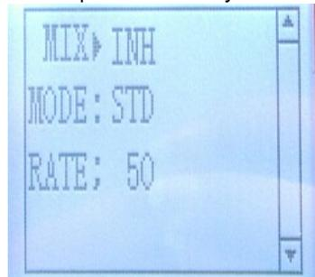
4. Press the button key Enter, the value stops flashing, the setting is finished now.
