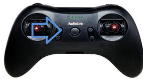
Yaw stick to the right, F121 turns clockwise
