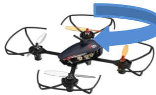
Yaw stick to the right, F121 turns clockwise
