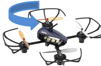
Yaw stick to the left , F121 turns anticlockwise
