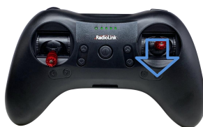
Pitch stick downward, F121 moves backward
