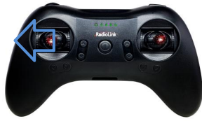
Yaw stick to the left , F121 turns anticlockwise
