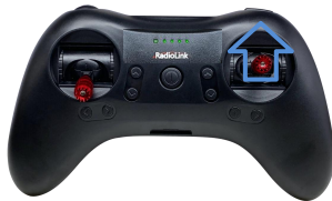
Pitch stick upward, F121 moves forward
