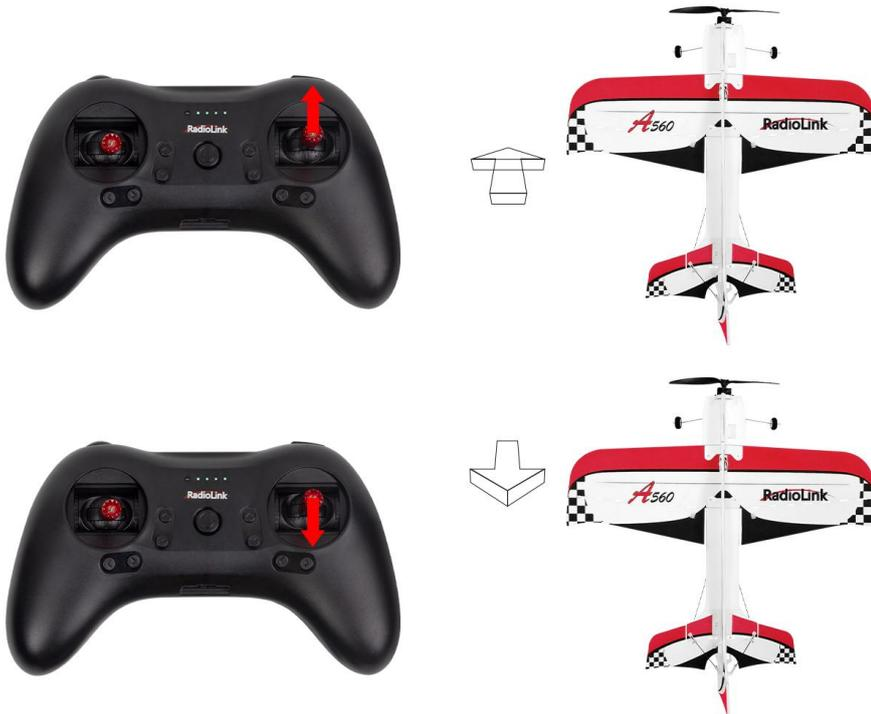
When the aircraft is vertical, toggle the rudder joystick(CH4) to control the aircraft moving (anti)clockwise.
