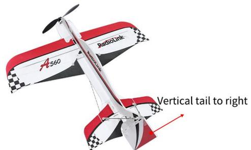
In manual mode, operate the joystick of the transmitter. If the movement of the control surface of the corresponding channel is reversed, enter the setting page of the transmitter to adjust the transmitter phase of the corresponding channel.
