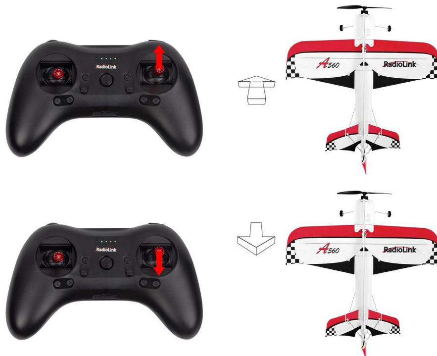
When the aircraft is vertical, toggle the rudder joystick(CH4) to control the aircraft moving left or right.
