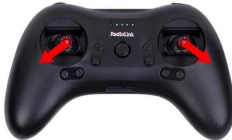
**Note:** When using a non-RadioLink transmitter, if the attitude calibration is unsuccessful when pushing the left stick (left and down) and the right stick (right and down), please change the direction of the channel in the transmitter. Make sure when pushing the joystick as above, the value range of channel 1 to channel 4 is:
