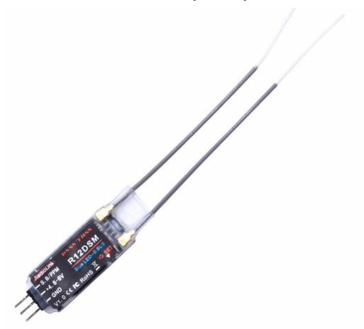
Radiolink R12DSM, 2.4G 12 channels receiver, DSSS and FHSS hybrid dual spread spectrum, 2.5 gram weight, SBUS and PPM signal support, use for Radiolink transmitters AT9, AT9S, AT10 and AT10II, is the best choice for racing drone.
