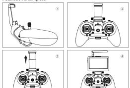
5. To remove the holder from the T8S transmitter, please take out the T8S from the bottom of the holder. Do not take out the holder from the position where the monitor is clamped to avoid damaging the holder.
