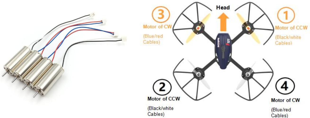
\* Motors installation can be skipped as the whole F121 is already assembled by factory default. If any of the motors is worn out and needs to be replaced, it's essential to identify the correct motor rotation.
