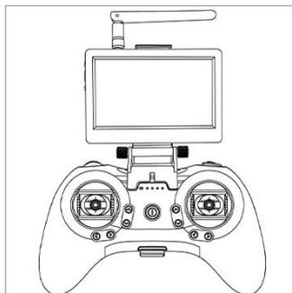
4. Install the holder on the T8S transmitter as shown above, and the installation is complete.
