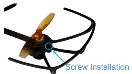
**Note** After the installation of the four propeller protectors, double confirm if they are leaning or slightly shake F121 to see if they drop. If they are crooked or drop, repeat the above steps to ensure the well installation.
