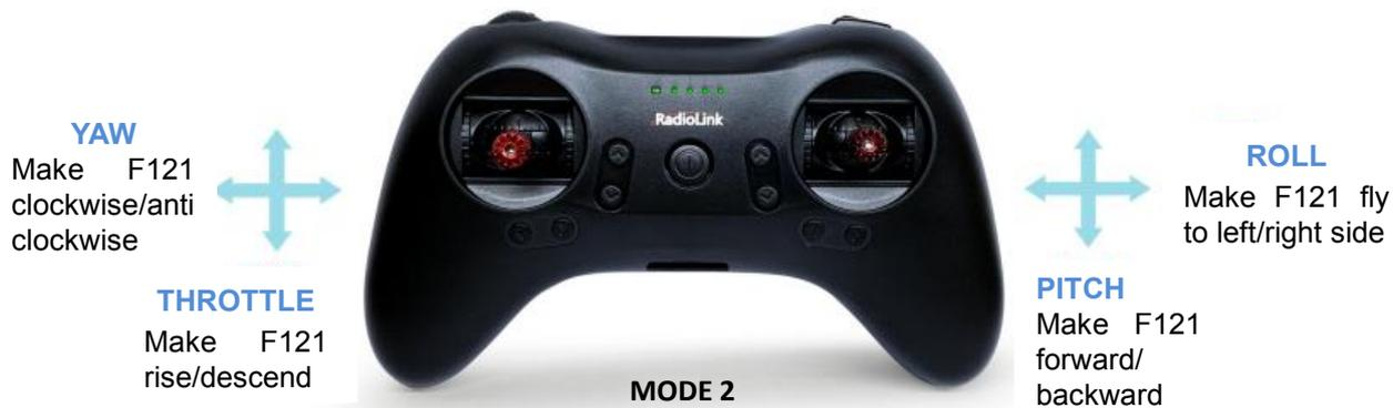
**Note** If it's the transmitter from other brands used with RadioLink F121, make sure that the receiver should be SBUS signal output supported. Once the receiver is installed on the mini drone, the phase of the throttle should be reversed while the other three channels normal and the CH5 should be set with a 3-way switch. Servo phases of transmitters from other brands should be set according to the actual situation.
