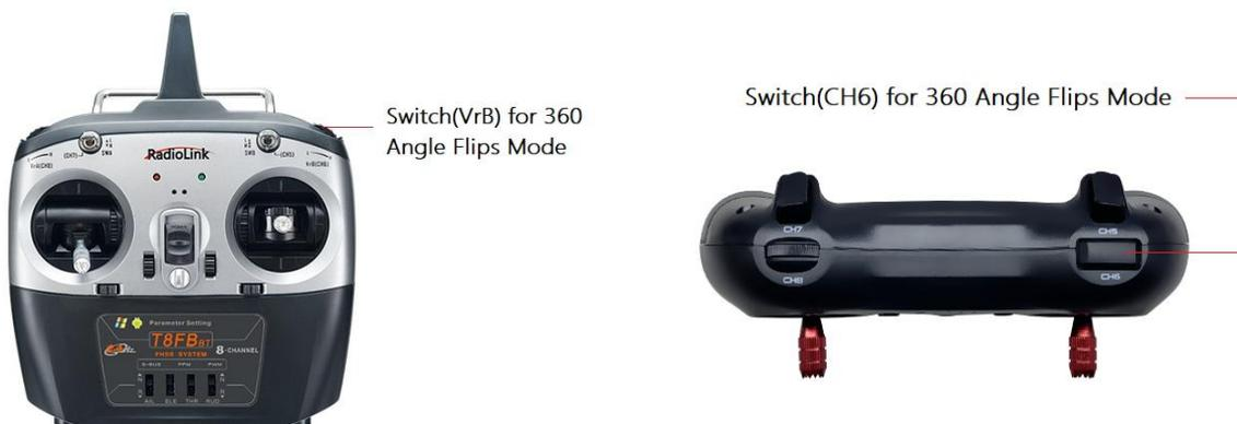
When the transmitter is T8S, press the CH6 switch twice continuous and then push the aileron or elevator stick. If push the aileron stick to the left, the F121 will roll 360 degrees to left. If push the aileron stick to the right, the F121 will roll 360 degrees to right. If push the elevator stick upward, the F121 will roll 360 degrees forward. If push the elevator stick downward, the F121 will roll 360 degrees backward.
