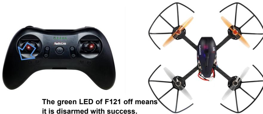
*Throttle on right (Mode 1):* With right joystick at bottom, toggle the left stick to the left and hold this position for 3 seconds till the green LED of F121 is off.
