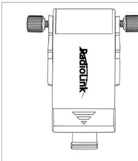
3. Use the two red screws to twist through screw holes on both sides of the holder in a clockwise direction. Be careful not to tighten the screws at this time. After adjusting the angle of the holder, you can tighten the screws to stabilize the holder.
