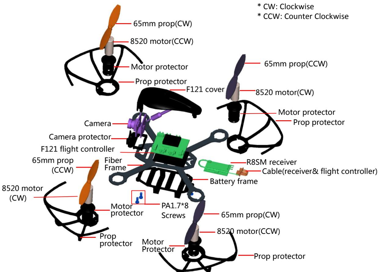
\*There are screws packed with F121 to ensure the firm installation of the propellers protector to the F121 frame even with collision. Pilots can fix them on as necessary.
