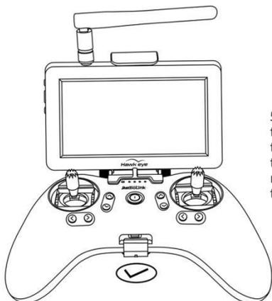
5.To remove the holder from the T8S transmitter,please take out the T8S from the bottom of the holder.Do not take out the holder from the position where the monitor is clamped to avoid dammaging the holder.
