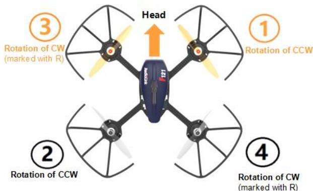
When the installation is done, make sure the four motors are vertical to the aircraft frame. Adjust them to vertical positions if necessary, otherwise F121 may not flight successfully.
