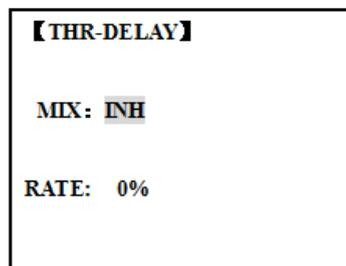
The THR-DELAY function is used to slow the response of the throttle servo to simulate the slow response of a turbine engine. A 40% delay setting corresponds to about a one-second delay, while a 100% delay takes about eight seconds to respond. This function may also be used to create a “slowed servo” on a channel other than throttle. This is accomplished by plugging the desired servo (Ex: gear doors) into CH3 (THR), throttle into an auxiliary channel such as 8, and then using some creative mixes.
