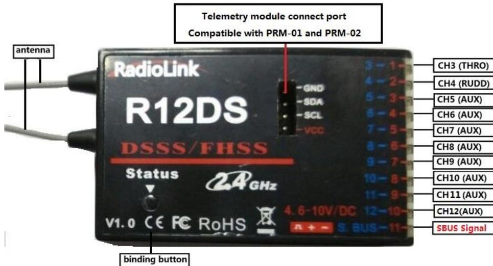
SBUS signal working mode:
