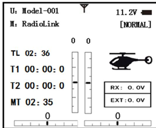
Find telemetry information: under BASIC MENU, select RECEIVE, presses PUSH to enter, you can find the telemetry info, shown as below. RX is receiver voltage, EXT is external voltage. Also temperature and engine speed (EXT, TEMPERATURE, RPM, and GPS all need telemetry sensor). RSSI is signal strength, NULL is for no signal, and 0 is for max. Connection of telemetry sensor: sensor of EXT, TEMPERATURE, RPM, GPS can connect one by one with the receiver port DATA.
