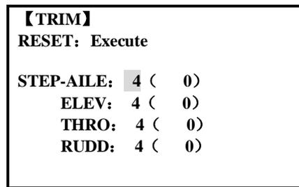
The AT10II has digital trims which are different from conventional mechanical trim sliders. Each TRIM LEVER is actually a two-direction switch. Each time the TRIM LEVER is pressed, the trim is changed a selected amount. When you hold the TRIM LEVER, the trim speed will increase. The current trim position is graphically displayed on the start up screen. The TRIM submenu includes two functions that are used to manage the trim options.
