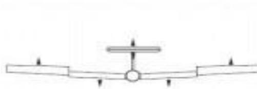
BUTTERFLY simultaneously moves the flaps, twin ailerons and elevator, and is usually used to make steep descents or to limit increases in airspeed in dives. Separate two BUTTERFLY settings are available. (CRI1/CRI2)
