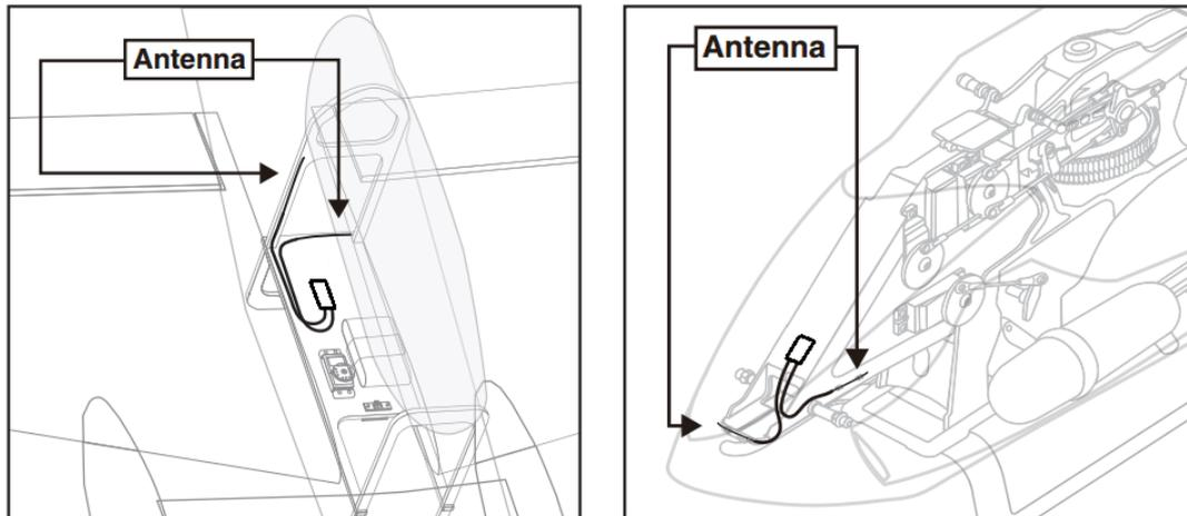
③ Antennas should be kept away from metal conductor and carbon fiber at least half inch away and no over bending.
