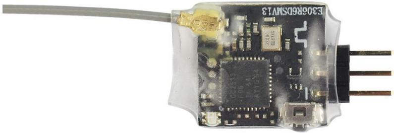
Radiolink R6DSM, 2.4G 10 channels receiver, DSSS and FHSS spread spectrum working synchronously, 1.5 gram weight, SBUS and PPM signal support, use for Radiolink transmitters AT9, AT9S , AT10 and AT10II, is the best choice for racing drone.
