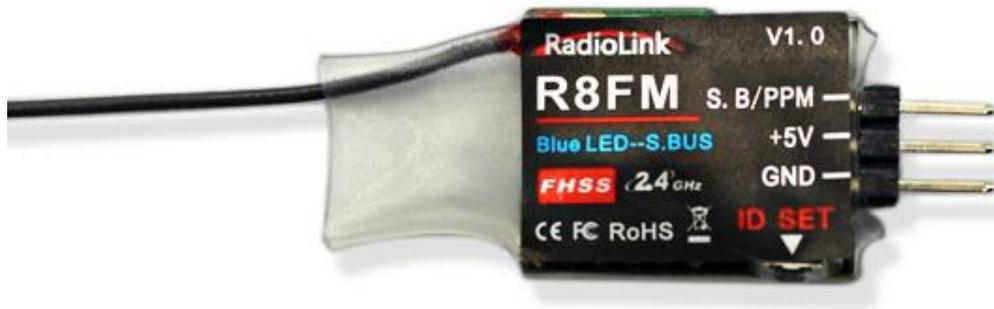
Radiolink R8FM, 2.4G 8 channels receiver, 2.5-gram weight, SBUS and PPM signal support, use for Radiolink transmitter T8FB, is the best choice for racing drone.
