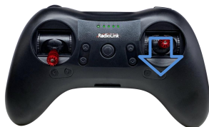
Pitch stick downward, F121 Pro moves backward
