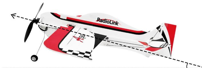
(2) Push the left stick (left and down) and the right stick (right and down) as below and hold more than 3 seconds. The green LED flashes once mean the calibration completed. It is also normal for the control surface to swing or the motor to rotate once at this time.
