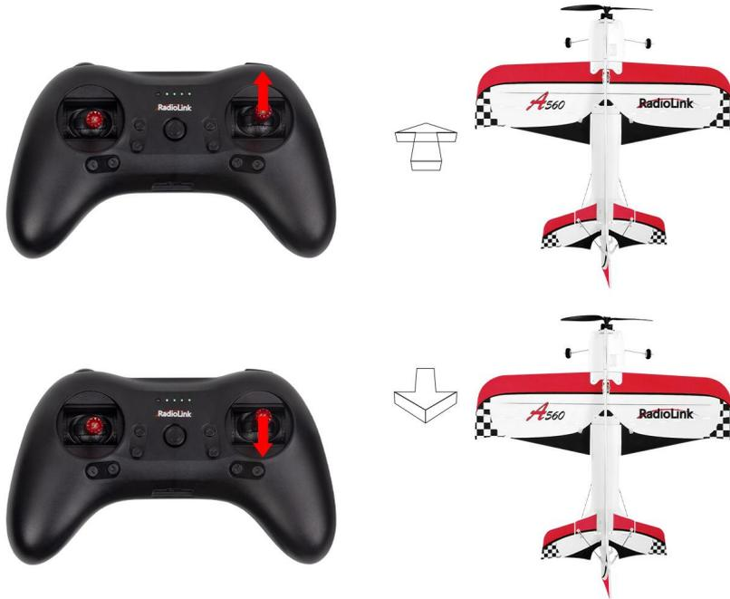
When the A560 is vertical, toggle the rudder joystick(CH4) to control the A560 moving (anti)clockwise.
