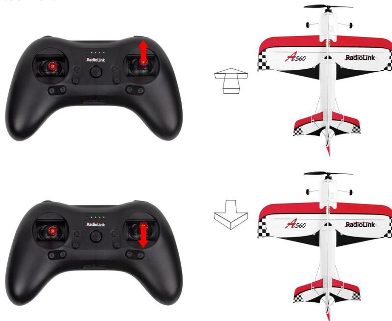
When the A560 is vertical, toggle the rudder joystick(CH4) to control the aircraft moving left or right.
