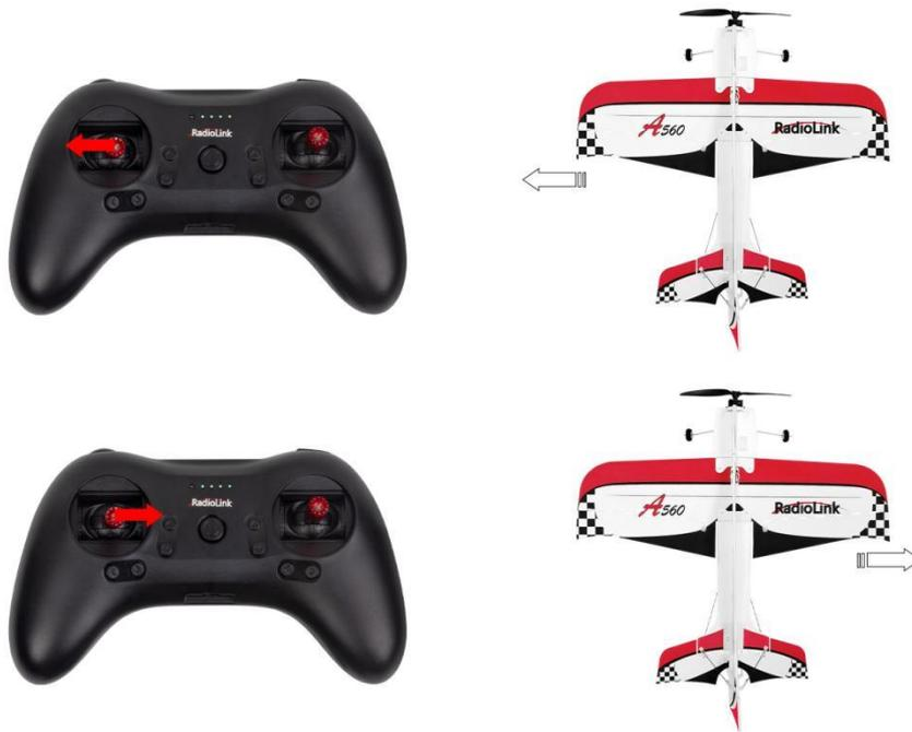
If the throttle joystick is toggled upward, the A560 climbs upwards at a vertical attitude. If toggled downward, the A560 descends at a vertical attitude.
