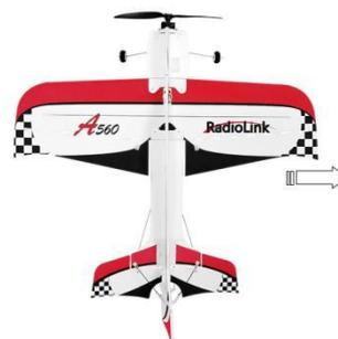
When the A560 is vertical, toggle the elevator joystick(CH2) to control the A560 moving forward or backward.
