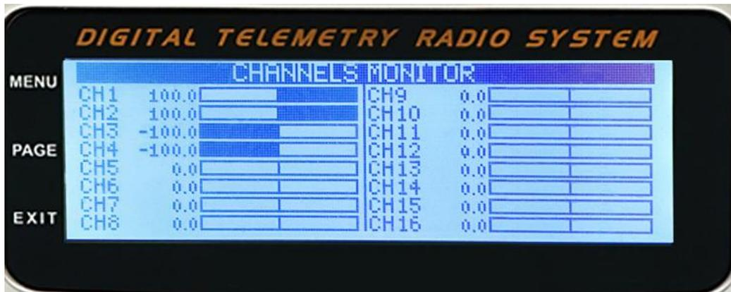
CH1 2000  $\mu$ s (opentx +100), CH2 2000  $\mu$ s (opentx +100)
