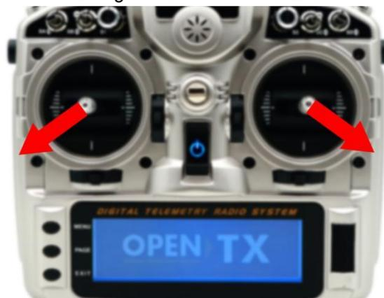
**Note:** When using a non-RadioLink transmitter, if the attitude calibration is unsuccessful when pushing the left stick (left and down) and the right stick (right and down), please change the direction of the channel in the transmitter. Make sure when pushing the joystick as above, the value range of channel 1 to channel 4 is:
