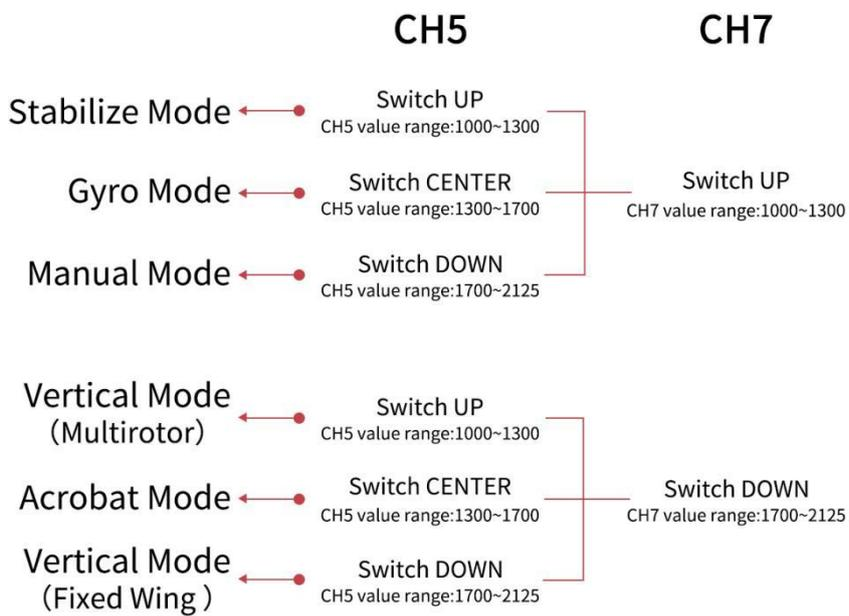
Take RadioLink AT9S Pro transmitter as example. Flight modes are set by CH5(3-way switch SWC) and CH7(2-way switch SWD) as below.
