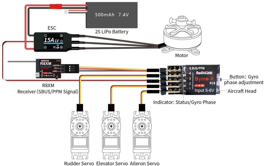
Channels on Byme-A V2.0 flight controller: CH1-Aileron, CH2-Elevator, CH3-Throttle, CH4-Rudder, S.BUS/PPM-connect to receiver, SBUS/PPM signal supported.
