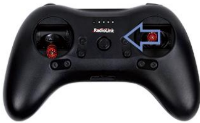
Roll stick to left, F108 fly to the left side
