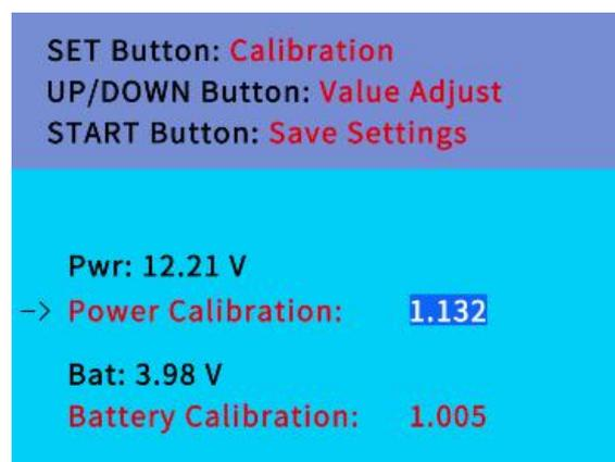
4. The calibration of the CB86-PLUS charger includes power supply voltage calibration and battery voltage calibration. Calibrate the power supply voltage first, and then calibrate the battery voltage. Please refer to the following calibration steps:
