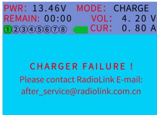
The main reasons for this warning are usually: abnormal input power supply, abnormal battery status, abnormal charger hardware etc.. Power off and restart the charger to exit this warning page, and then perform specific troubleshooting.
