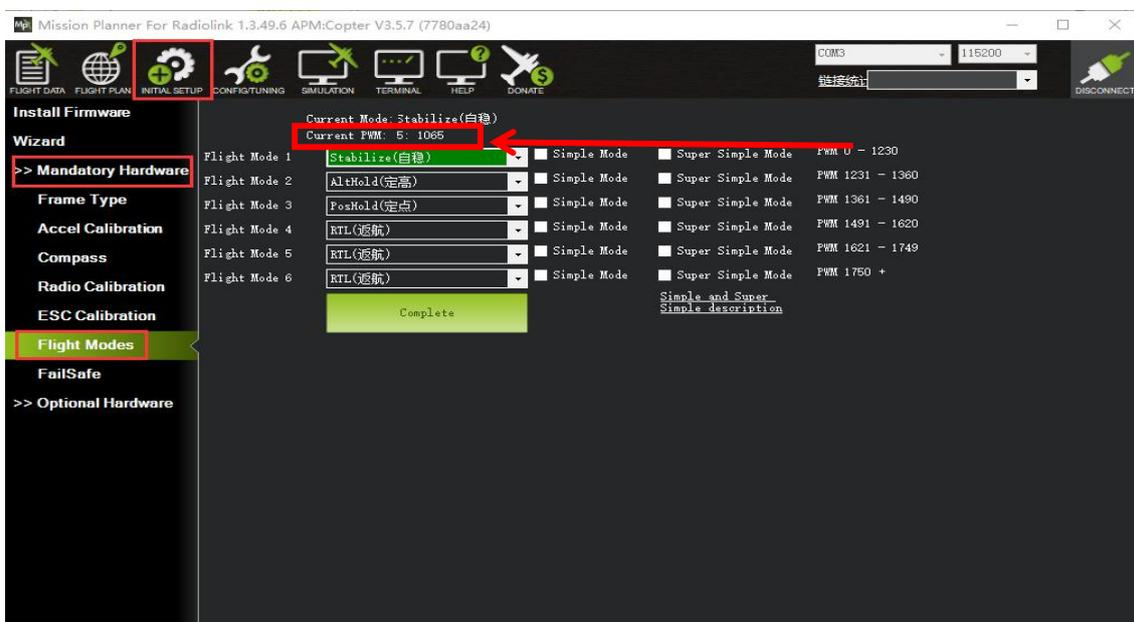
When setting the PWM value on transmitter, the corresponding PWM value on MP will change accordingly. Each flight mode has the PWM range and when the value is within, it means the current mode is set. Meanwhile, the selected mode on MP will turn dark green. That is, turning the dial on the transmitter to modify the RATE to make sure the corresponding PWM value on MP is within the range. Flight mode 2/3/4/5/5 can be set as the same way.
