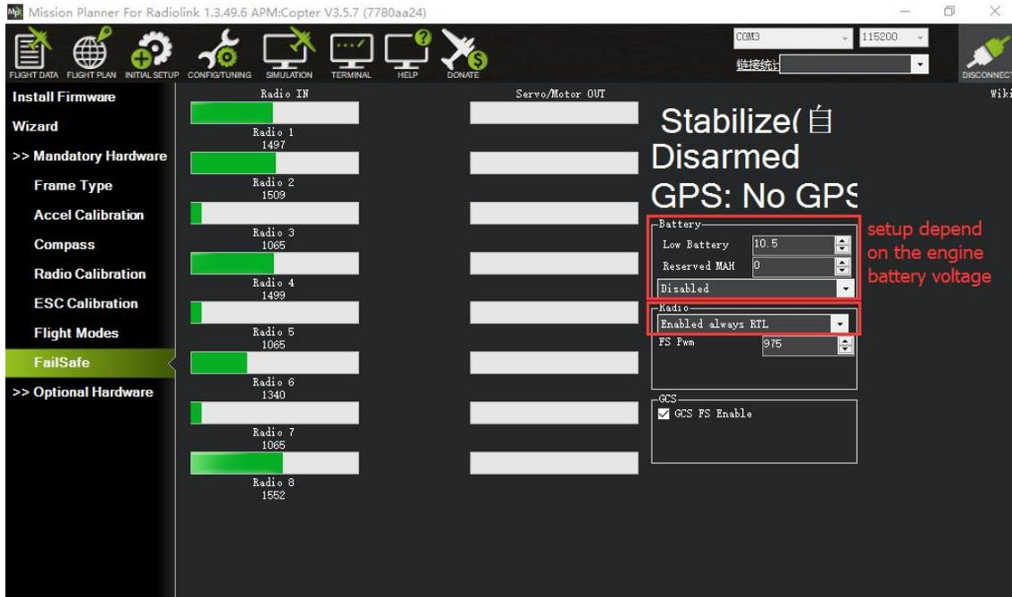
There are different parameters setting such as throttle PWM, battery voltage to enable Mini Pix failsafe function. When the set parameter is reached, eg. If the throttle PWM value or the voltage is lower than the value set, then the failsafe is enabled and the aircraft will take corresponding action such as Return to launch(RTL), Continue to flight and Landing. To ensure the aircraft safety, RTL is normally set as the action following failsafe enabled.
