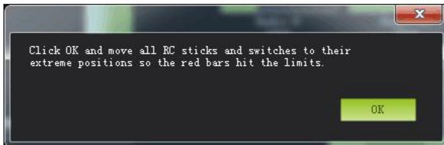
Joysticks can be calibrated as following , both (Ch1 to Ch4) are pushed to the limits(up/down/left/right)
