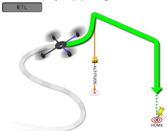
RTL Mode works with GPS, which is indispensable to locate before changing to this Mode. The Mode commands the aircraft to return "HOME" where it takes off. Therefore, "HOME" should always be the place that the GPS locates where the aircraft actually takes off, without obstacles and far away from crowds.
