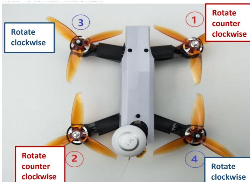
**Note:** Never install the props when setting parameters of aircraft to ensure the safety.
