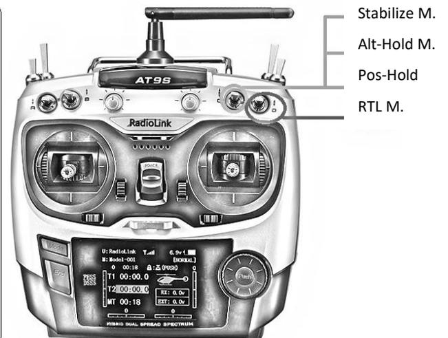
4. When flight mode 1 in MP is Stabilize, the first ATTITUDE on transmitter should be set as Stabilize and the corresponding parameters setup in MP should be set as below:
