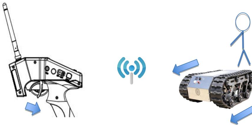
Throttle mix steering setup completed, both tracks moves forward when pulling the throttle
