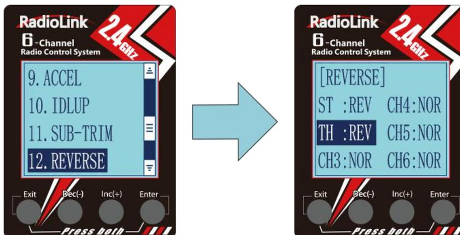
\* If the throttle reverse is correct, skip this throttle reverse setup.
