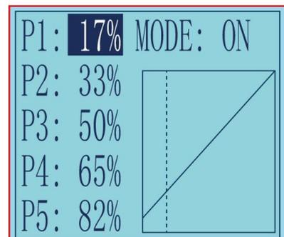
2. Press “Dec(-)” or “Inc(+)” button to select curve points 1~5 for curve point adjustment that you want, from the graph you will clearly see the changes you have made.
