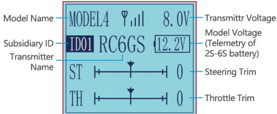
When you power on the transmitter, LCD screen shows Model Name, Transmitter Name, Transmitter Voltage, Steering Trim, Throttle Trim, Model Voltage, Subsidiary Model ID, Returned Signal.
