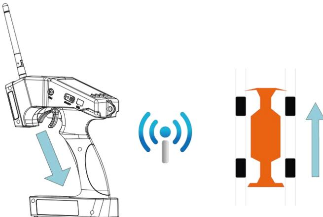
When pulling the trigger, the car moves forward
