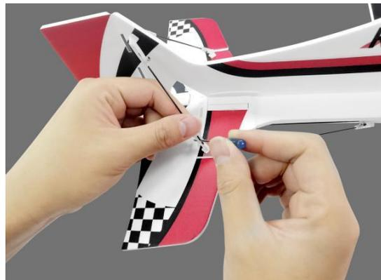
③ when packing the fuselage in the bag, please keep all drawbars and support rods parallel to the fuselage to avoid damage to the drawbar/rod caused by improper placement.
