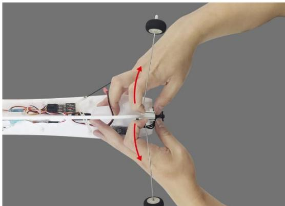
② When disassembling the drawbars or support rods, please put the screwdriver in the middle gap of the clasp, and then pry it.
