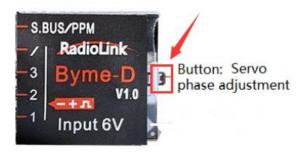
Note: Make sure attitude calibration is complete before changing the servo phases. Byme-D will identify the installation position(above/bottom of the aircraft) to automatically adjust the gyro direction.
