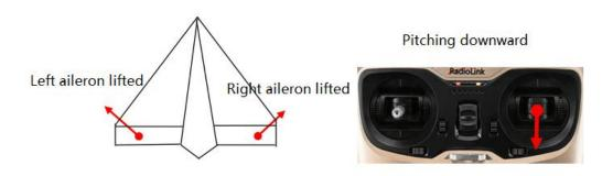
When the movement direction of the aileron is inconsistent with the joystick, please adjust the servo phase through the buttons on the front of Byme-D. Please do not change any settings of servo direction on the remote control at this time.
