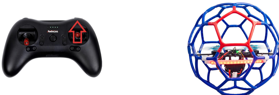
Pitch stick upward, LD-B20C moves forward
