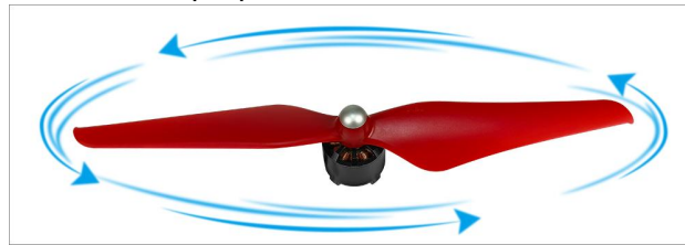
CCW propellers (counterclockwise rotation)
