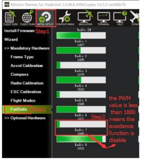
You can check the avoidance effect of the Ultrasonic Sensor SU04 after all the parameters have setup and connect the sensor SU04 to the PIXHAWK.
