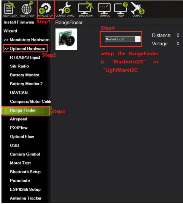
After the Range Finder setup, reconnect the flight controller and back to this Range Finder parameter setup menu, it will show the detection distance details means all the Range Finder parameters setup successful.
