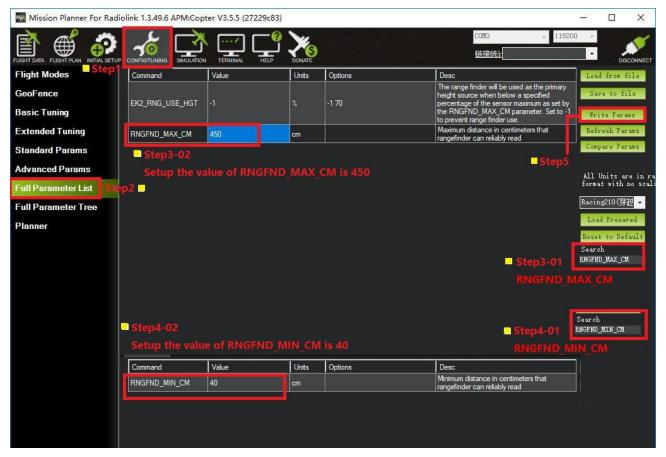
**RNGFND\_MAX\_CM** means the max detection distance that can identify at the AltHold Mode.
