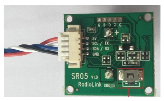
Press this button to change the direction of obstacle avoidance, it will rotate 45 degrees clockwise when press the button once.
