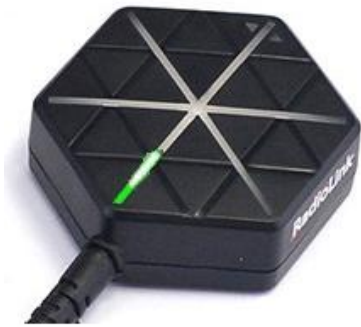
the green LED near antenna will on when SE100 power on
