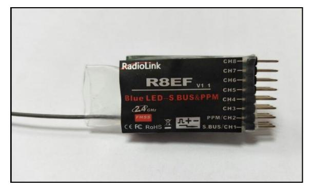
Radiolink R8EF, 2.4G 8 channels receiver, S-BUS, PPM and PWM signal support, use for Radiolink transmitter T8FB.
