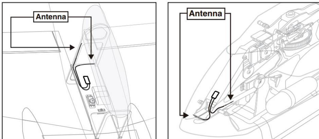
4. The antennas must be kept away from conductive materials, such as metal and carbon. at least a half inch. The coaxial part of the antennas does not need to follow these guidelines, but do not bend it in a small radius.
