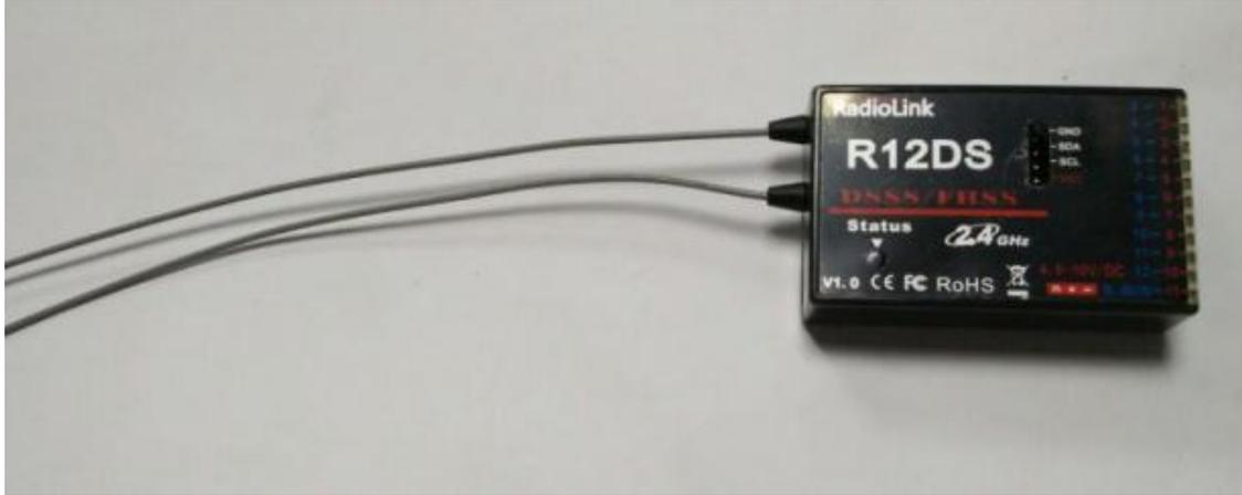
Radiolink R12DS, 2.4G 12 channels receiver, DSSS and FHSS spread spectrum working synchronously, compatible with Radiolink transmitters AT9, AT9S, AT10 and AT10II(AT9, AT9S, AT10 can upgrade to 12 channels just upgrade by firmware, you can download the firmware from our website: <http://radiolink.com.cn/doce/at10upgraded.html>, AT10II is default 12 channels).
