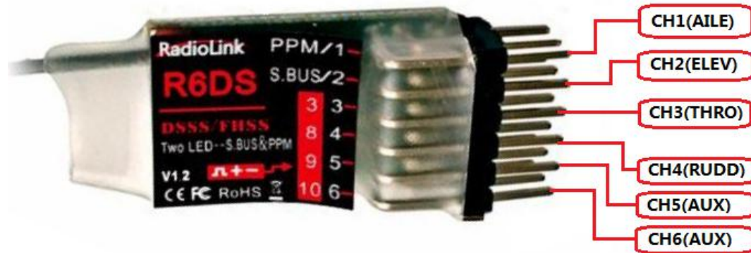
PWM signal working mode, 6channel
